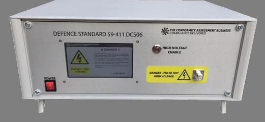
The Conformity Assessment Business Model DCS06 Test Generator has been designed to operate with it's complimentary injection clamp to fully meet the pulse requirements of DCS06 when tested in to a 5 $\Omega$  load. It operates from an intuitive touch screen interface and has full phase synchronisation up to 800 Hz input frequency with 1 degree steps. It has been designed with future revisions of the test standard in mind.
